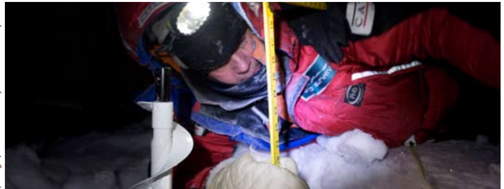
The ice team drill into the ice to measure its thickness.
